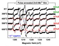
**EPR:** Mn<sup>2+</sup>-c grows for *T* > 400 °C → crystallization of the amorphous phase + GBs diffusion
